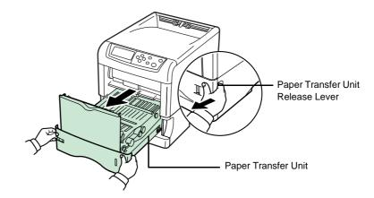
4 Open the rear cover and then the fuser cover, and remove the jammed paper.
